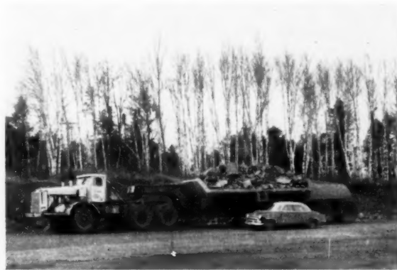
NEW GIANT OF THE MESABI is this 90-ton trailer truck developed by Reserve with passenger car for size comparison.
